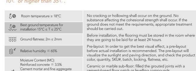
color, quantity, SKU#, batch, locking, flatness, etc. Ceramic or marble sub-floor: filled the grouted joints with a cement-based floor patch or levelling compounds.
